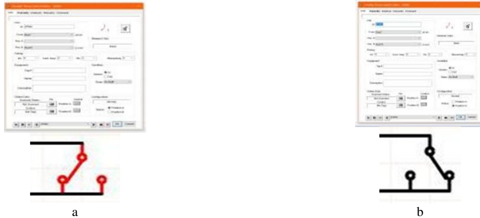
FIGURE 2. Symbols and Descriptions of Switches in Locked Position (A) and Released Position (B)
