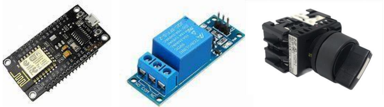
Figure 1. A. NodeMCU ESP8266 B. Relay C. Selector Switch
